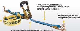
Ratchet handles with double pawl & locking action safety system to prevent slipping off the load
